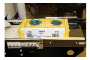
The conveyor on the front of the 44R will pull trays into the machine as space permits. The system controller will monitor the presence of trays and allow them to move forward by actuating stop pins located on the bottom of the conveyor.
