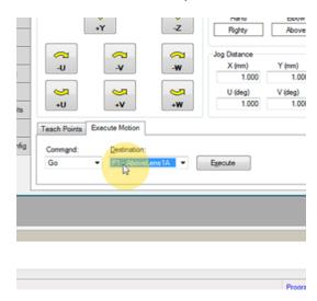
34. Remove the tray and calibration tools from Tray Position 1 and place in Tray Position 2 and repeat calibration steps
