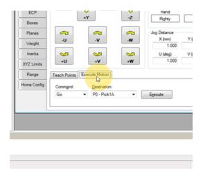
8. Select Point 01 (if machine operates left to right) or Point 23 (if machine operates right to left) from the Destination drop menu
